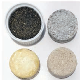
Mycelium swatches with added milk paint powder
