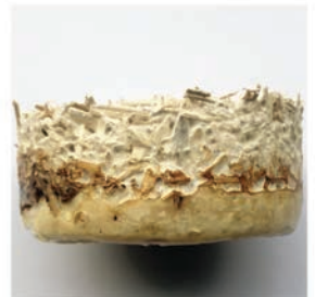
Testing latex and mycelium grown into each other
