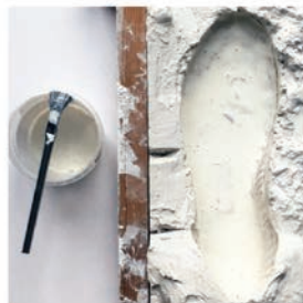
Final thick layer of latex before adding the mycelium
