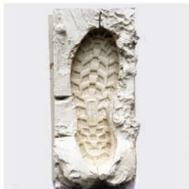
Plaster mould of outer sole
