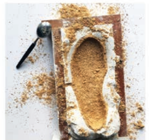
Adding grow material to latex layer in mould
