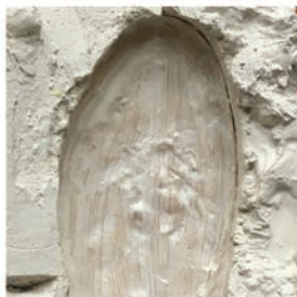
Layer by layer building latex outer sole
