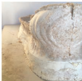
Finished latex/mycelium outer sole
