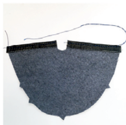
Pineapple leather cut, skived, folded, glued and sewn
