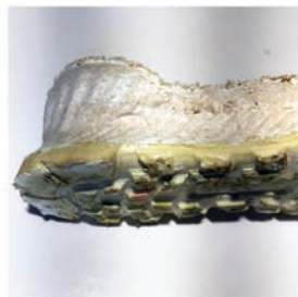
Finished latex/mycelium outer sole
